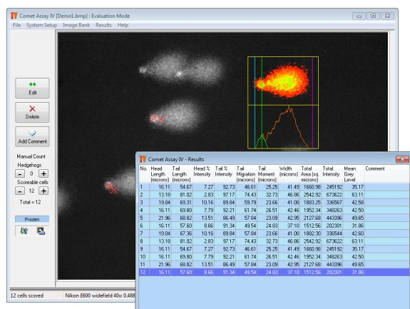
Measurements accumulated for each slide are viewable within a scrolling results window, which can be split from the main application and placed on a second screen in dual-monitor systems. The results window can also be hidden entirely for those wishing to score blind.
