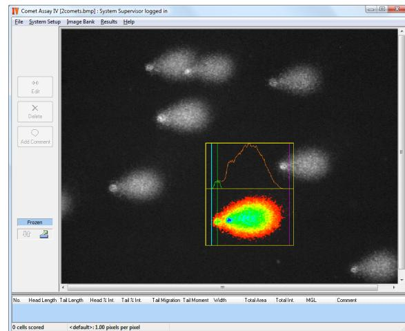
In addition to this, Comet Assay IV's **Hedgehog Counter** provides a simple mechanism for users to integrate 'hedgehog' cell counts with the rest of the measurement data.
