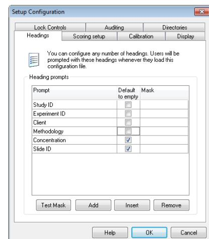
**Comet Assay IV**'s Save using headings feature makes it easy to organise your result files by using the heading entries to automatically define file and folder names. If you intend to use an **Oracle** database for secure storage of data, all heading entries will be saved to the database along with the corresponding result data.
